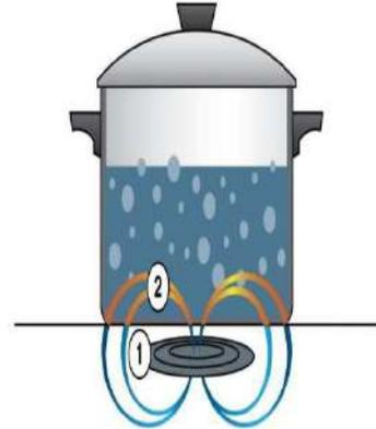
**Induction Cooktop/Cook stove:** An induction cooktop is a cooking surface that heats by transferring currents from an electromagnetic field located below the glass surface directly to the magnetic induction cookware placed above. Unlike thermal conduction, it heats this cookware directly without the need for a flame or burner. Because there is no heating of a separate element, an induction cooktop can heat cookware faster than any other medium.
