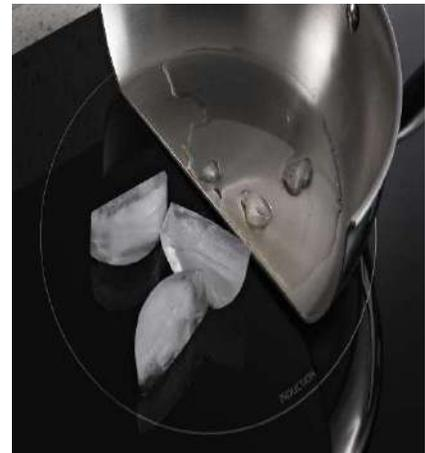
An induction Cooktop/hob contains a coil of copper wire underneath the ceramic plate, and when a cooking pot is placed on top an alternating electric current is passed through it. The resulting oscillating magnetic field induces a magnetic flux, producing an eddy current in the ferrous pot, which acts like the secondary winding of a transformer. The eddy current flowing through the resistance of the pot heats it.
