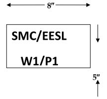
In the above format, **W** is the ward number and **P** is the pole number. The base shall be painted with yellow color while as the marking shall be done with black color. The dimensions of the pole marking as shown above shall be **8"x 5"**.
