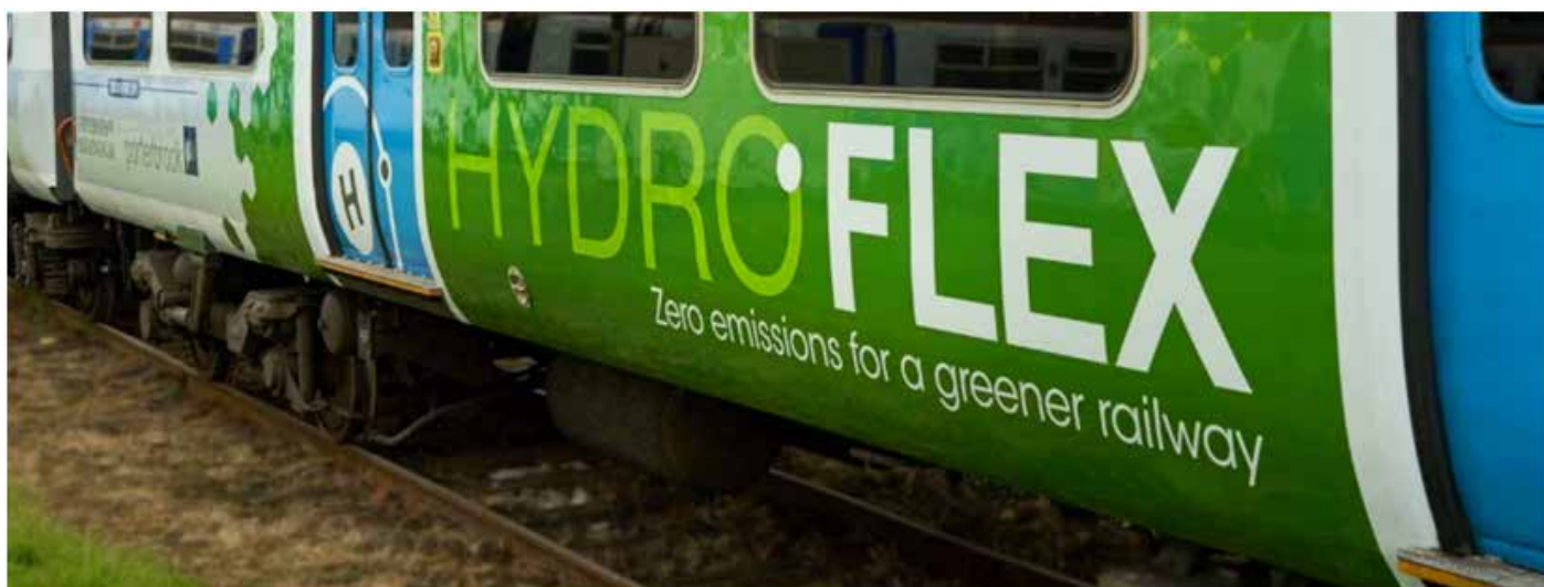
The 30-year-old Diesel Multiple Unit HydroFLEX vehicle has been converted to Hydrogen fuel cell power
