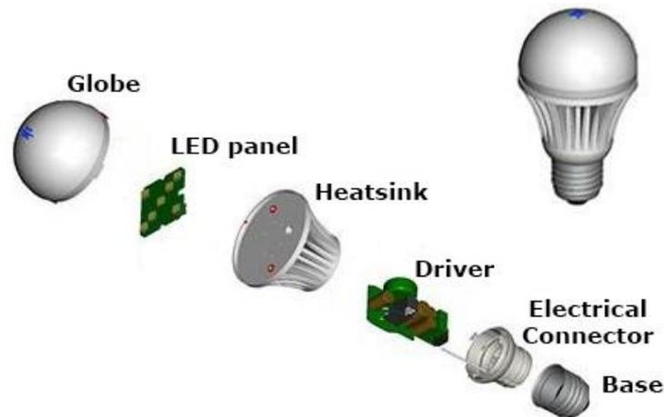
Figure 2: Components of a standard LED lamp<sup>3</sup>
